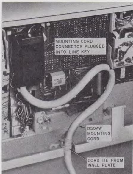
Fig. 15—D50AW Mounting Cord Connected to Wall Set
