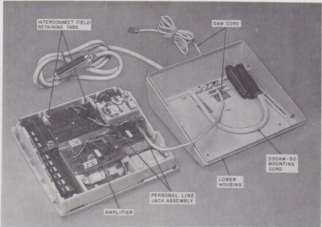
Fig. 50—Basic Satellite Desk Set Disassembled
