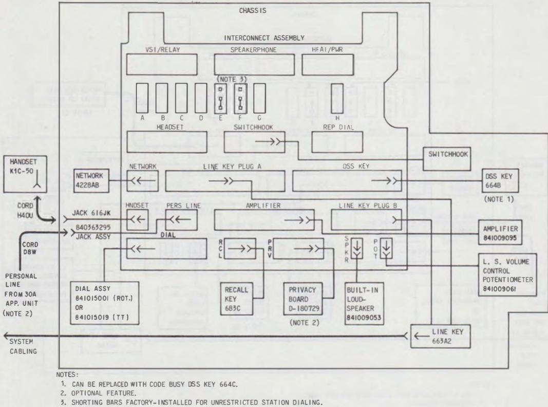
Fig. 44—Block Diagram of Basic Satellite Wall Set
