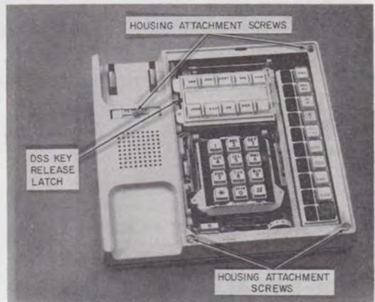
**Fig. 49—Basic Satellite Set, Faceplate Removed**
