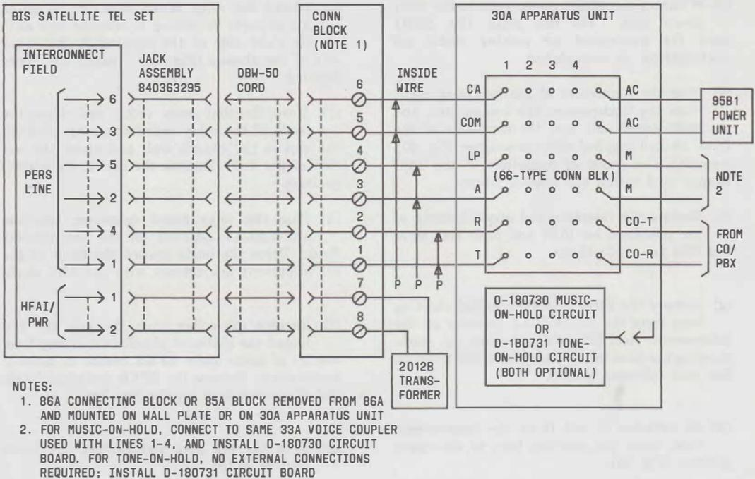
Fig. 39—Personal Line Connections for BIS Satellite Sets
