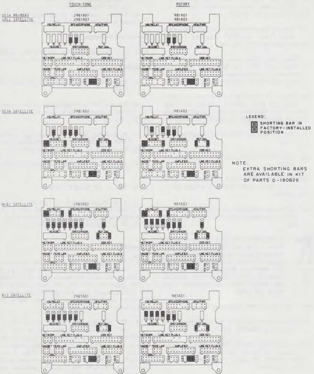
Fig. 34—Interconnect Fields Showing Factory Positions of Shorting Bars
