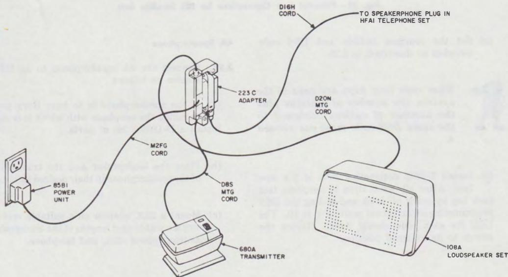
Fig. 40—4A Speakerphone Installation and Connections
