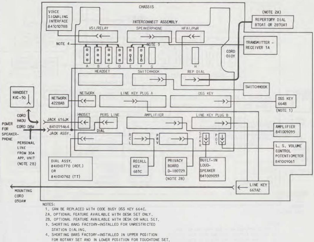
Fig. 45—Block Diagram of BIS Satellite Set
