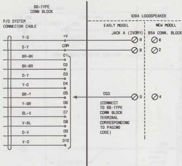
Fig. 25—Paging Connections Using 66-Type Connecting Block
