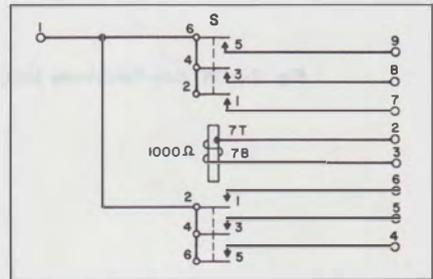
**Fig. 1—3A Key Telephone Unit, Intercommunicating Signaling Circuit**
