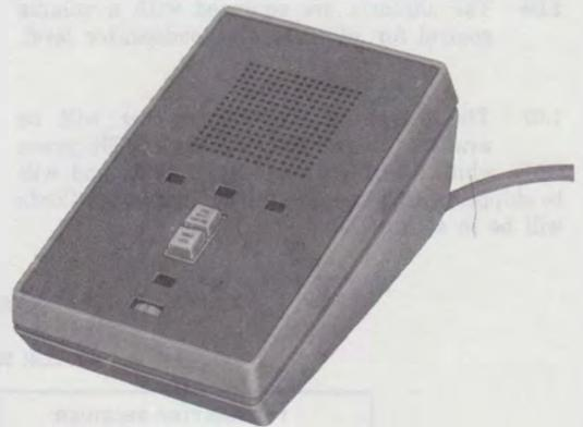
B. 2B TRANSMITTER-RECEIVER (THREE-PATH)
