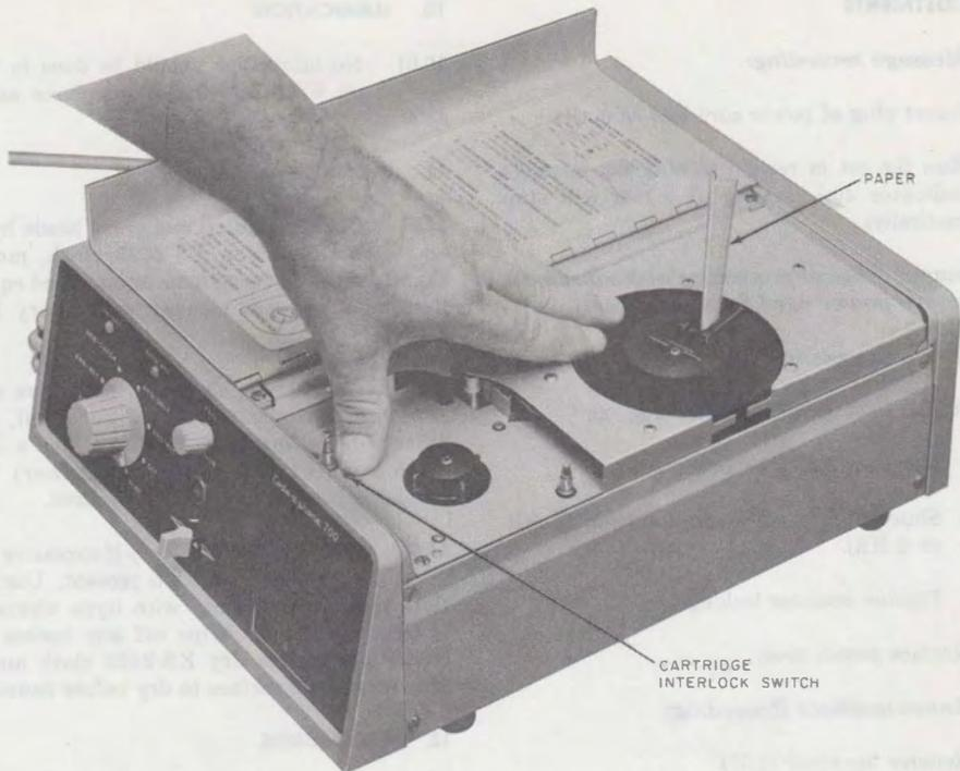
**Fig. 7—Resetting “0” Registration on Message Indicator Dial**
