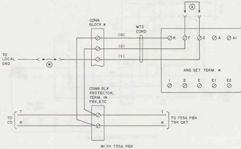
Fig. 6—KS-19245, List 1 Telephone Set Connections (Sheet 2 of 3)
