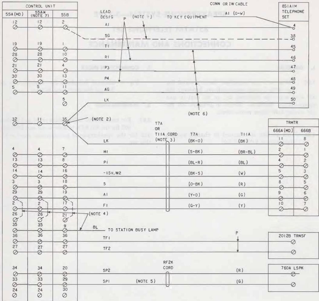
Fig. 1—851A1M Telephone Set, Connections to 3-Type Speakerphone System
