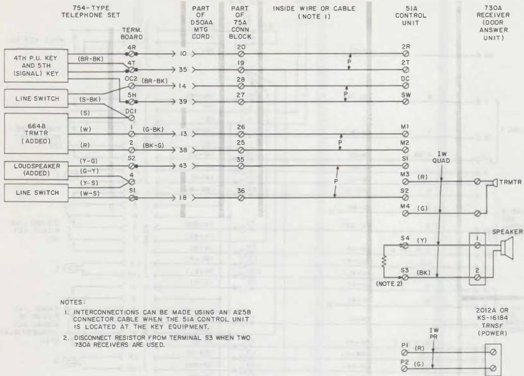
Fig. 4—754-Type Telephone Set, Connections to 1A Home Interphone System
