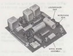
Fig. 4—Amplifier Gain Controls
