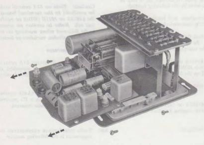
Fig. 5—Wiring Board Assembly Removal
