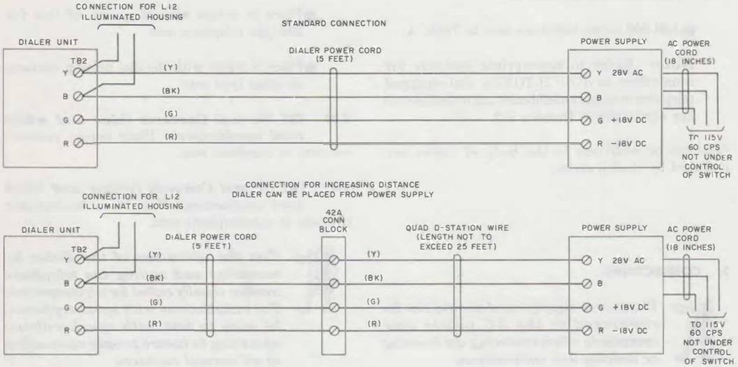
**Fig. 1 — KS-1954 Dialer, Power Supply Connections**
