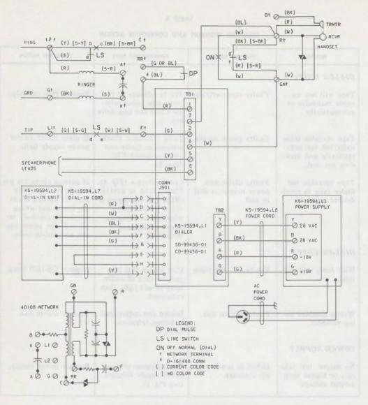
Fig. 2—Typical Installation Layout, KS-19594 Dialer
