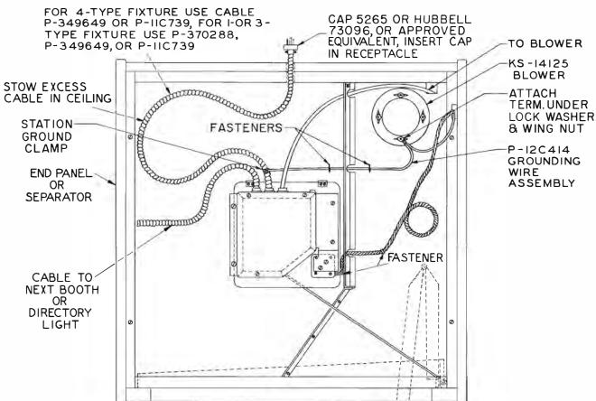
Fig. 4 — Typical Installation for 3-way Receptacle
