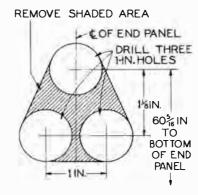
Fig. 11 — Hole for 2D Fixture
