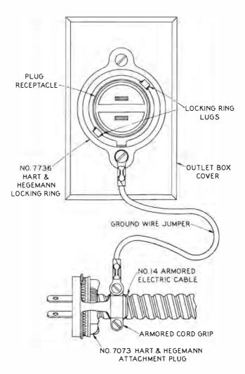
Fig. 5 — 2-wire Receptacle and Plug
