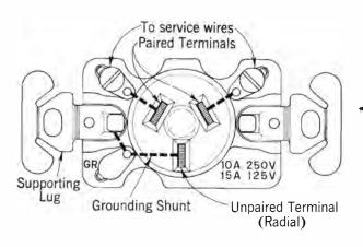
▼ Fig. 1 — 3-wire Flush-type Receptacle with
