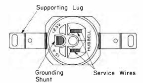
Fig. 2 – 3-wire Grounding-type Convenience ► Outlet, Hubbell No. 5261
