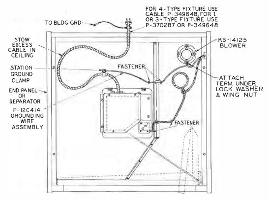
Fig. 6 - Typical 2-wire Cable Arrangement
