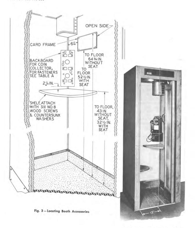
Fig. 2 - 11-type Booth with Plumb Line
