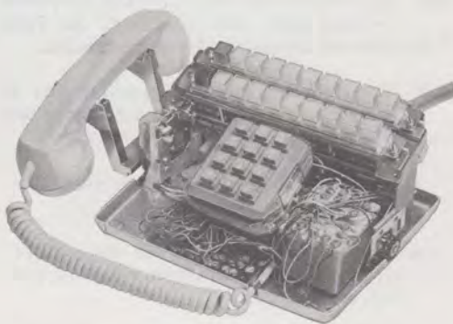
Fig. 2—2833-Type Telephone Set (Housing Removed)
