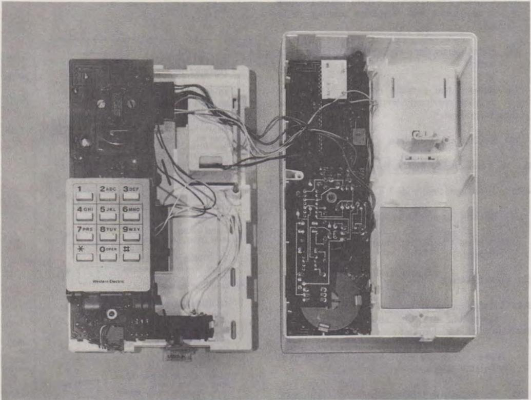
Fig. 5—5011T01A Telephone Set With Upper Housing Removed
