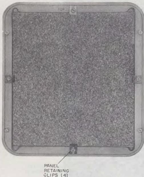
Fig. 4—Rear View of Frame With Panels Installed
