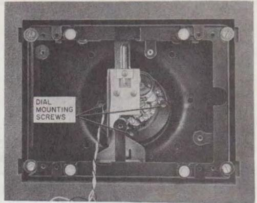
Fig. 6—Removing Dial
