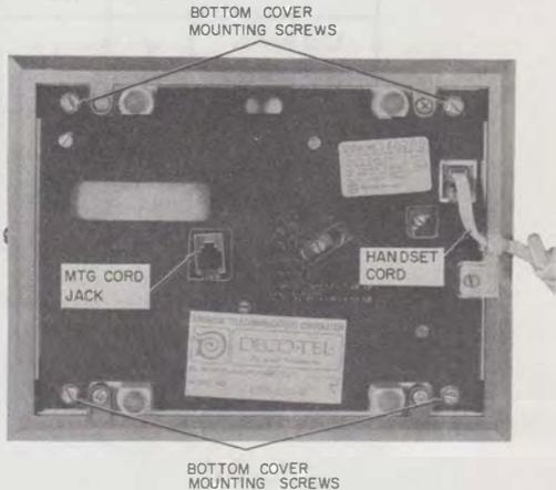
Fig. 4—Current Model Telephone Set, Bottom View
