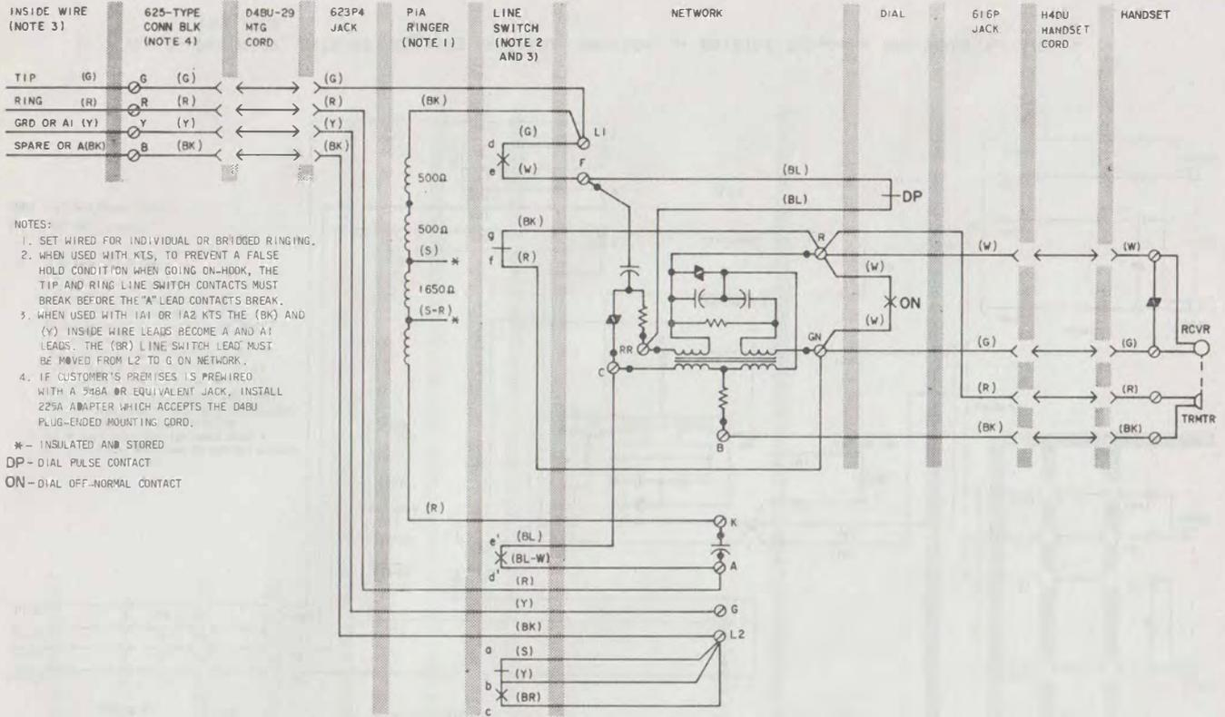
Fig. 9—881C102, 881C103, or 881C104 Telephone Set, Connections
