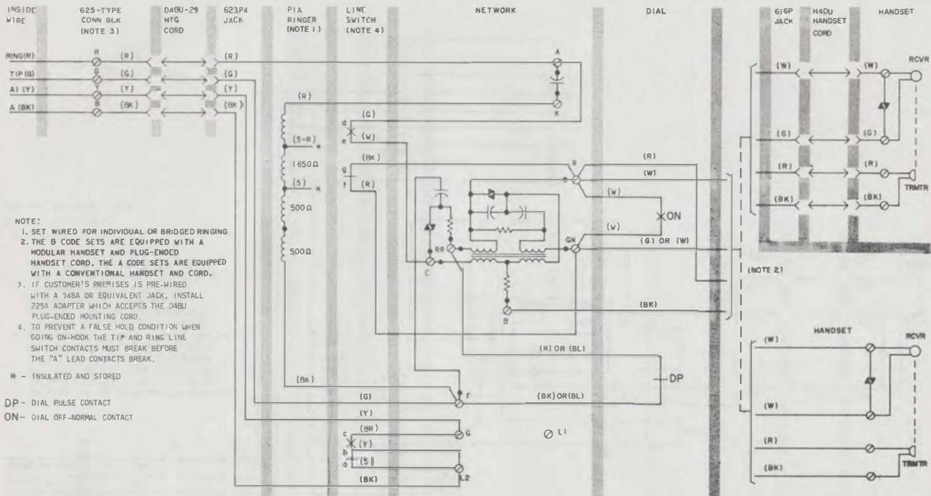
Fig. 8—881A102, 881B102, 881A103, 881B103, 881A104, or 881B104 Telephone Set Wired for 1A1 or 1A2 KTS
