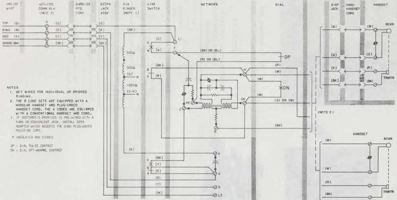
Fig. 7—881A102, 881B102, 881A103, 881B103, 881A104, or 881B104 Telephone Set, Connections
