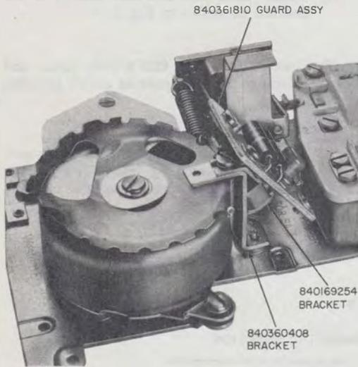
Fig. 4—Installation Location of Components to Add Polarity Guard Feature
