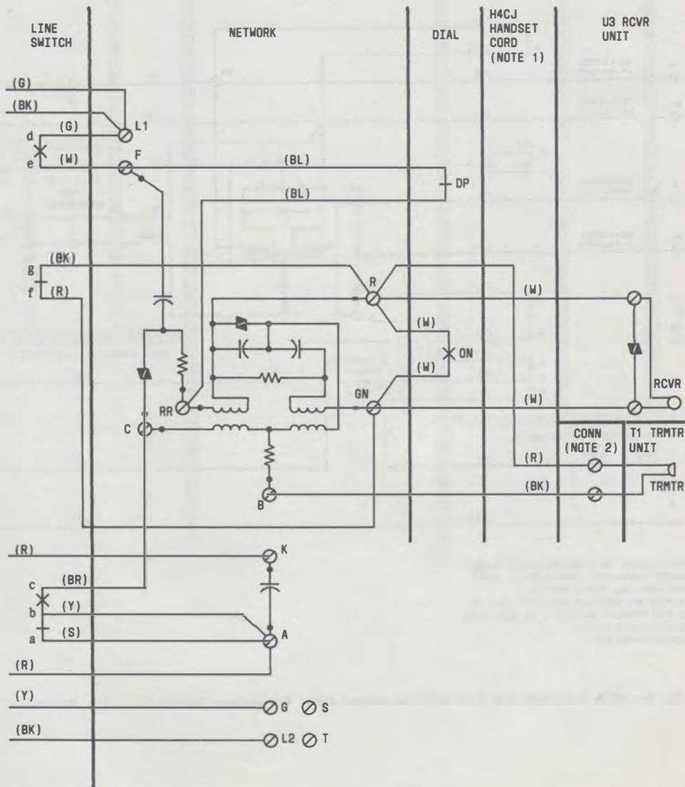
Fig. 8—581A Telephone Set Base With D-180778 Kit of Parts (Rotary Dial, Current Version) (Sheet 2 of 2)
