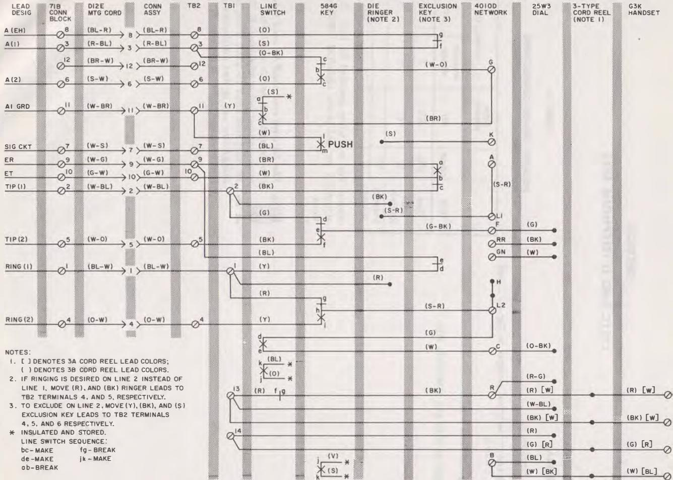
Fig. 1—1751C and D Telephone Set Connections With 25W3 (MD) Dial
