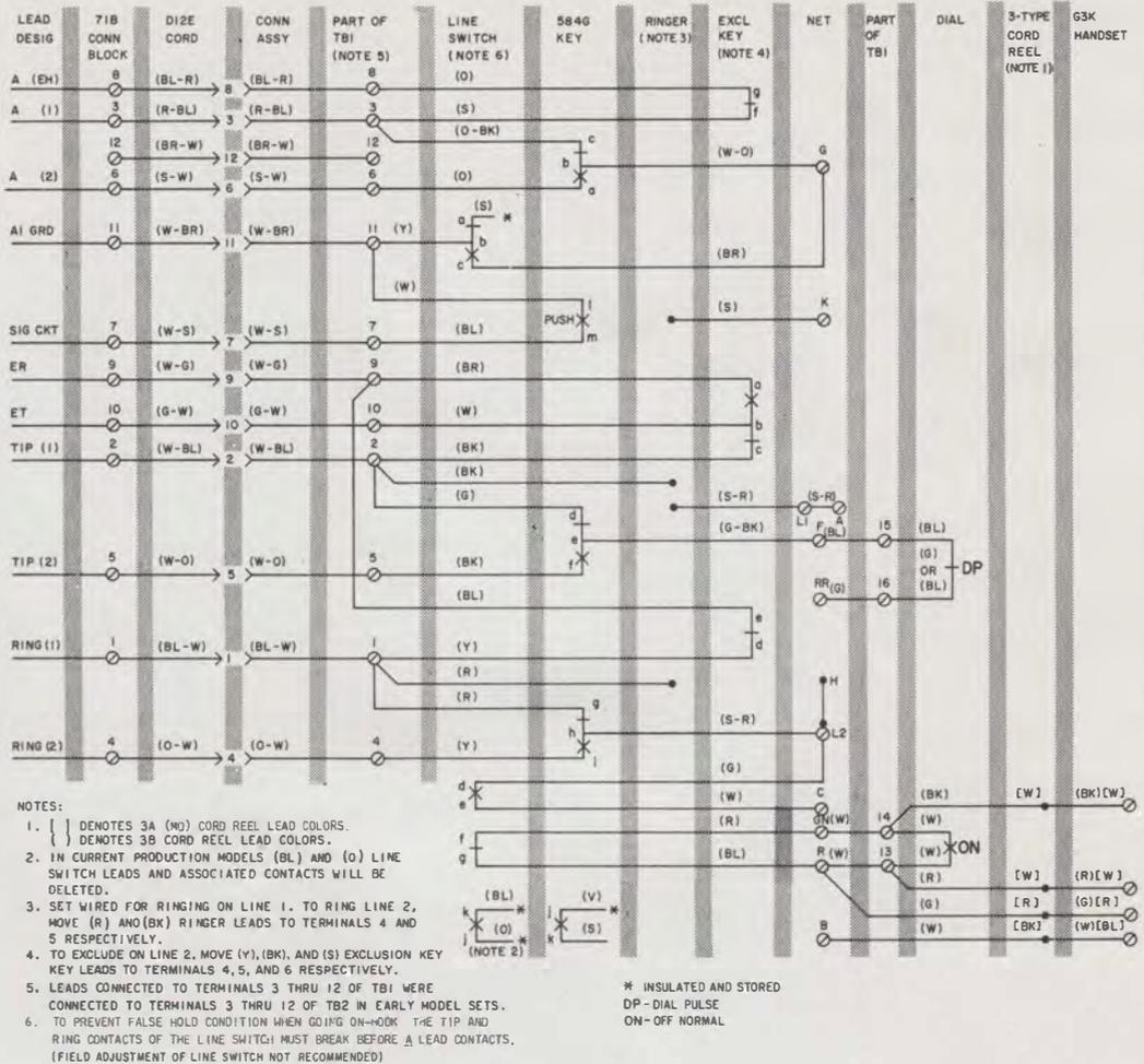
Fig. 2—751C and 751D Telephone Sets, Connections
