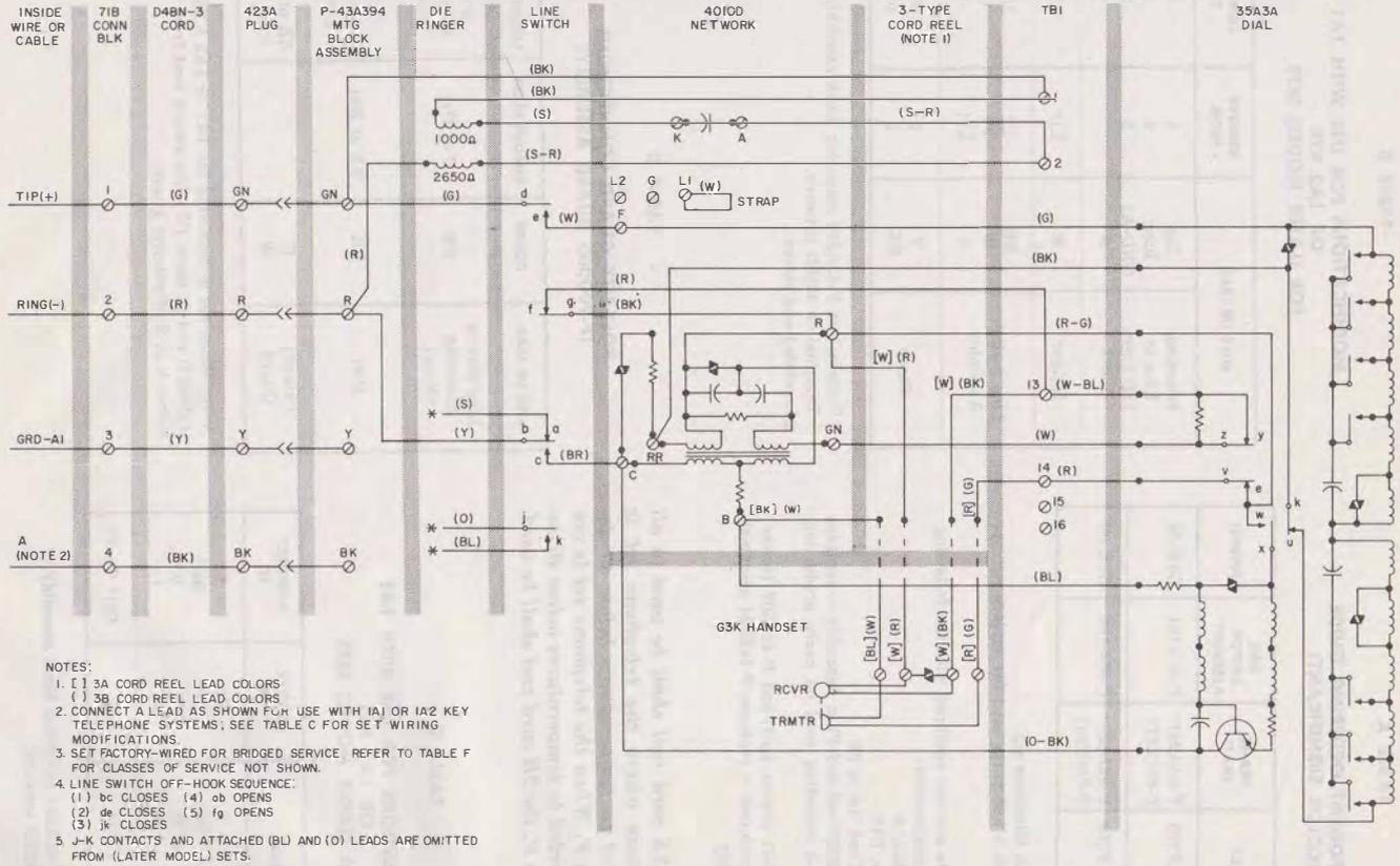
Fig. 5—2750-Type Telephone Set (Early Models)-Connections
