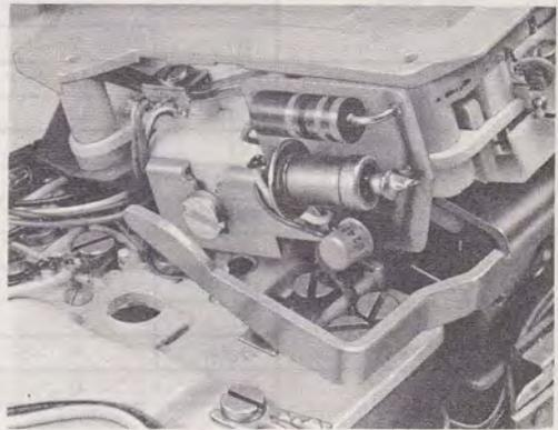
**Fig. 5—Polarity Guard Mounted in PRINCESS Telephone Set**
