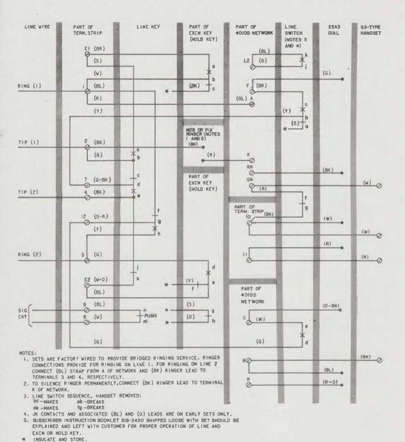
₱Fig. 2—1555B Telephone Set, Connections With 25A3 (MD) Dial
