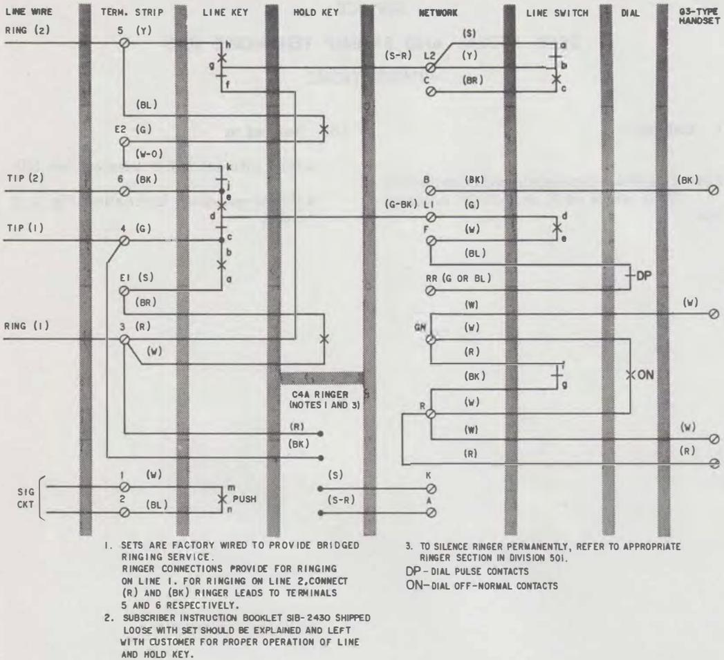
Fig. 1—555B (MD) Telephone Set, Connections
