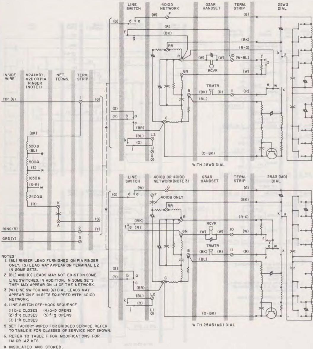
Fig. 3—1554B(MD) Telephone Set, Connections
