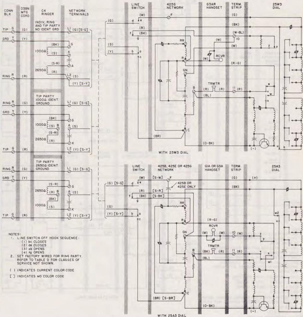
Fig. 2—1500D Telephone Set, Connections
