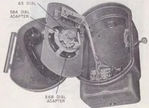
Fig. 2—525B (MD) Telephone Set (Dial), Inner Door Open
