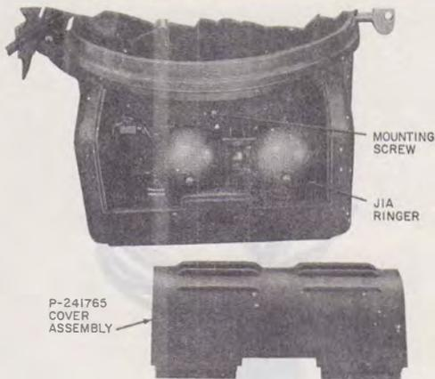
**Fig. 8—525 (MD)-Type Telephone Set, Cover Assembly Removed**
