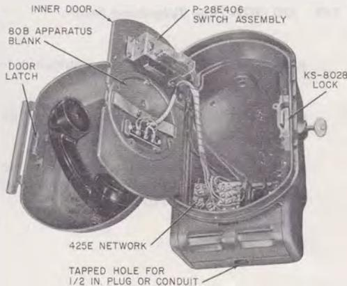
Fig. 1—525A (MD) Telephone Set (Manual), Inner Door Open
