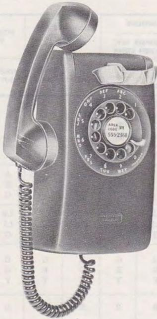
**Fig. 2—554- or 556-Type Telephone Set With Handset in Waiting Position**
