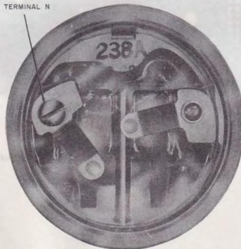
Fig. 7—238A Amplifier Showing Typical Terminal N Location
