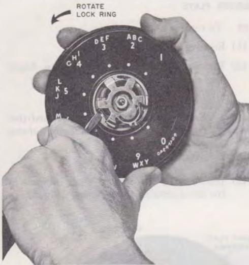
Fig. 7 — Lock Ring Removal
