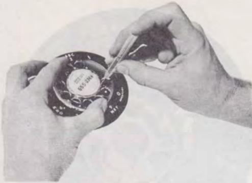
Fig. 4 — Removing Plastic Fingerwheel
