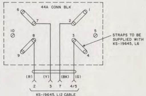
Fig. 29—KS-19645, List 6 Recorder Connector
