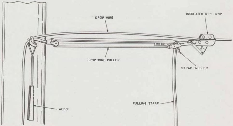
**Fig. 3—Tensioning Drop Wire**
