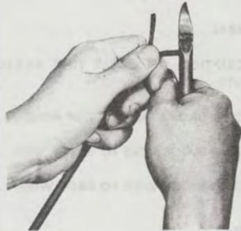
Fig. 3—Crushing Insulation
