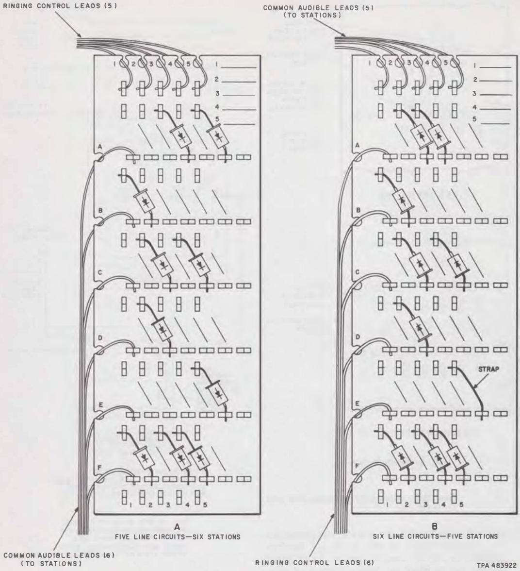
◆ Fig. 8—Wiring Arrangement and Diode Orientation ◆
