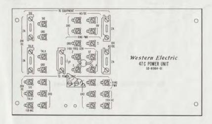
Fig. 3-Wiring Connections for 47C Power Unit
